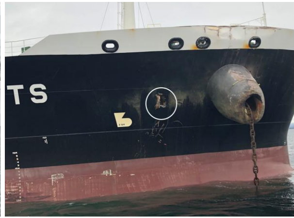
Figure 5: The hawsepipe and the damage sustained by Sola TS in the collision. The hole in the hull is marked with a white circle. Photo: The Norwegian Maritime Authority
